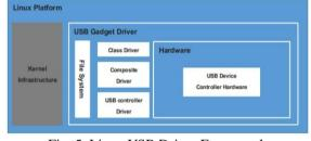
Fig. 5. Linux USB Driver Framework
